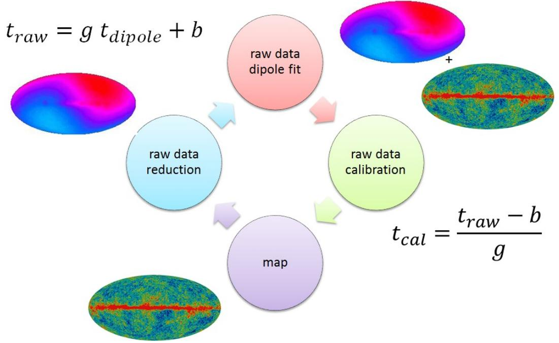
Figure 2: Iterative TOD calibration.
